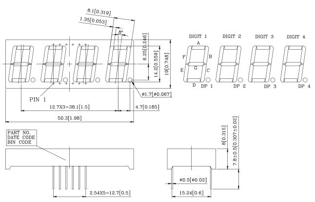
NOTES: 1.All dimensions are in millimeters. Tolerances are  $\pm$  0.25 mm (0.01") unless otherwise noted. 2.Pin tip's shift tolerance is +/- 0.4 mm.( suggest mother board pin hole  $\psi$ 1.0 mm )
