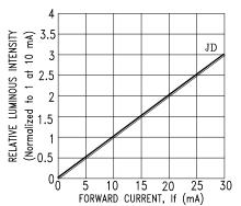
Fig3. Relative Luminous Intensity vs. DC Forward Current
